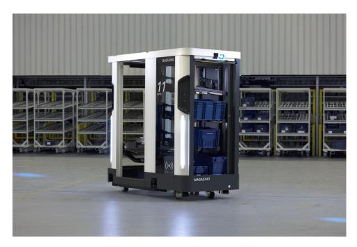
Image description: The SOTO robot autonomously brings several small load carriers from the central warehouse to the assembly line.
