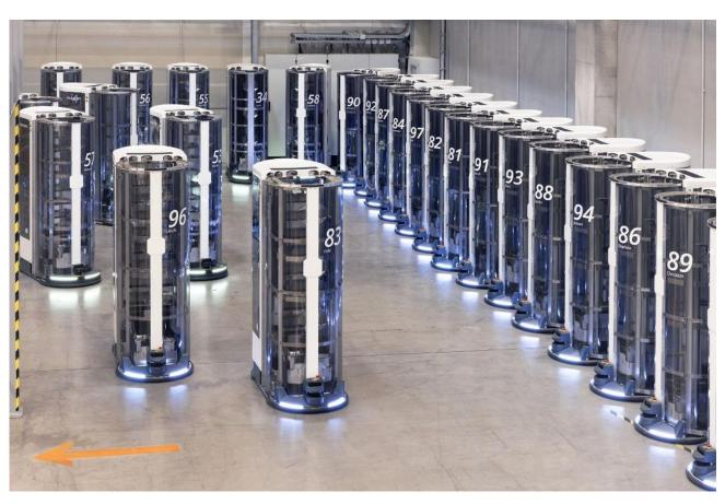
The mobile robot TORU autonomously transports, picks, and stows individual objects like shoe boxes."
