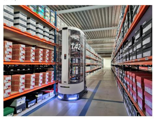
The robot TORU picks individual shoe boxes completely autonomously and thus supports the employees at Schuurman Schoenen in the warehouse. (Picture: Magazino GmbH)
